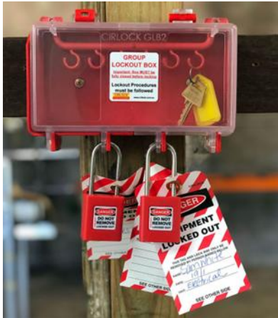
Image 6 – Example of a group lockout box
