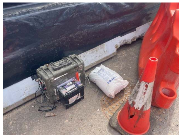
Photo 21: Vibration monitor on the southern site boundary
