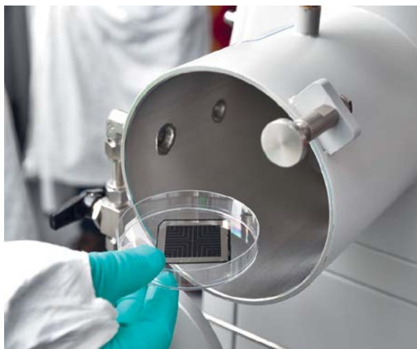
Removing a perovskite cell from a 'inert box', which protects the cell from moisture and other contaminants.
