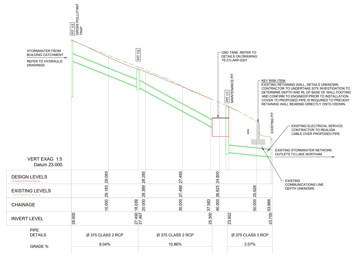
STORMWATER PIPE (NETWORK) LONG SECTION
