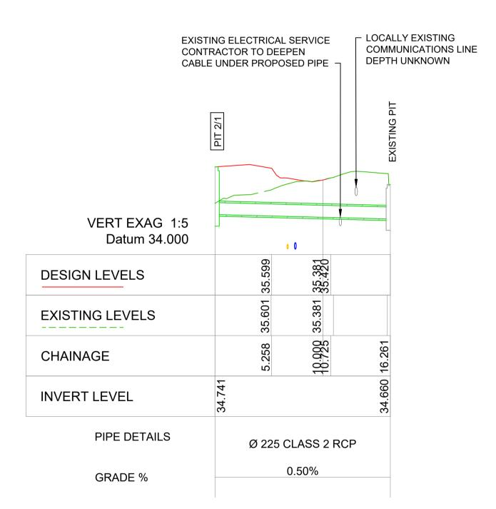
STORMWATER PIPE (ENTRY COURT) LONG SECTION
