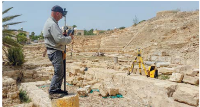
▲ Surveyor Guy Hazell geo-maps the location of granite columns that were part of the colonnade of the Roman road.
