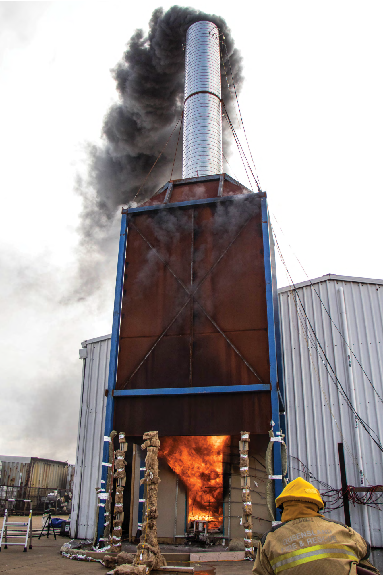
Cross Laminated Timber (CLT) fire test at UQ.
