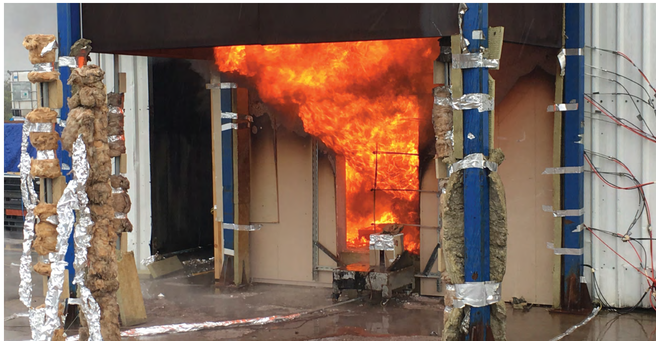
Fire Safety Engineering test on a cross laminated timber compartment.
