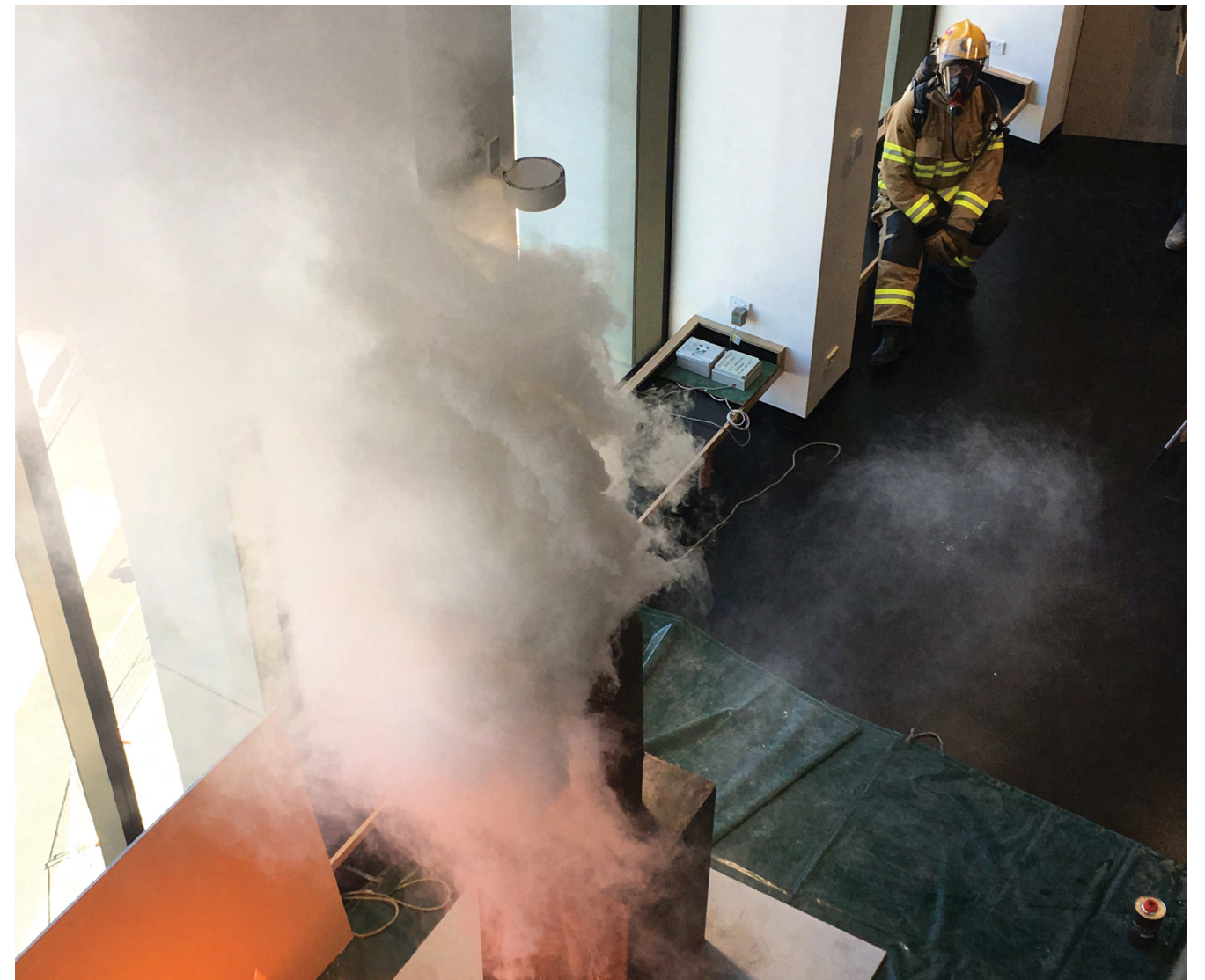
Hot smoke test at a university laboratory.
