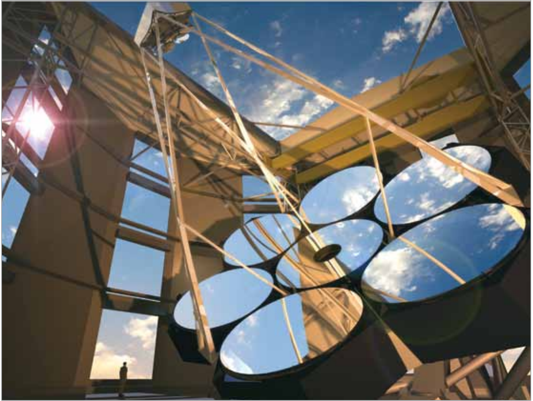
Figure 9: The proposed Giant Magellan Telescope will use seven 8.4-metre diameter mirrors to synthesise a single mirror some 22 metres in diameter. It is being proposed by an international consortium, which includes the Australian National University. (Source: Todd Mason, GMT Project.)
