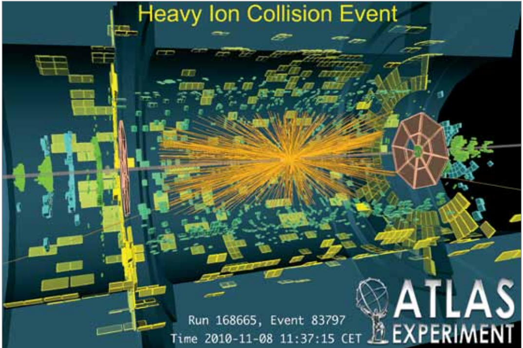
Figure 16. Reconstruction of a lead-lead collision recorded by the ATLAS experiment at the CERN LHC
