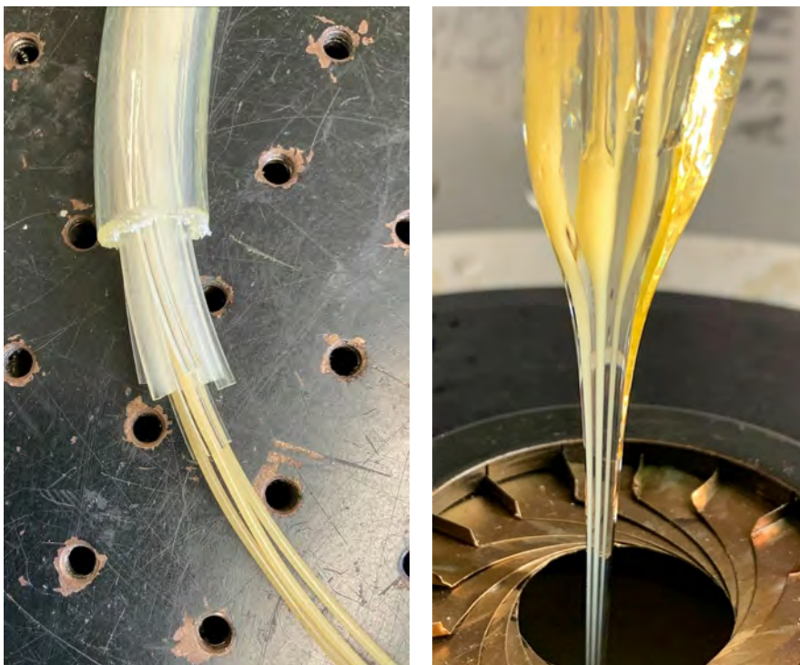
Figure 2. Drawing microstructured polyurethane fibre.
