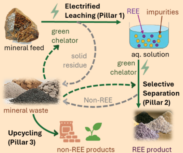
Conceptual schematic of a low-carbon platform for rare earth element extraction, combining electrified leaching, selective extraction using green chelators and electricity, and waste upcycling into higher-value by-products or extractant precursors.
