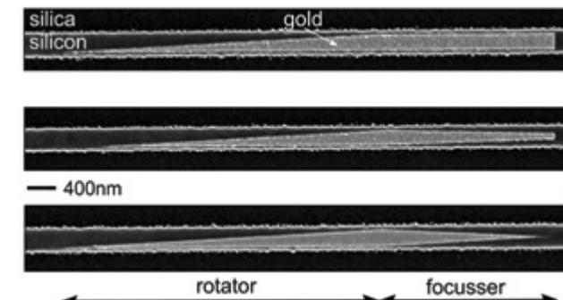
Scanning electron micrograph (top view) of silicon on insulator waveguides post processed with hybrid plasmonic waveguide circuits
