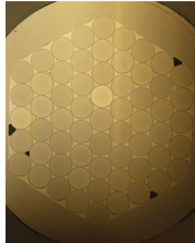
A ‘hexabundle’ which comprises 61 optical fibres fused into an imaging bundle. Hexabundles are used on astronomical instruments on large telescopes to take spatially resolved spectra of galaxies. This hexabundle is part of the Hector instrument.
