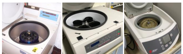
Centrifuges for a variety of uses including cell extract clarification
