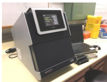
Circular dichroism, to explore structure and stability
