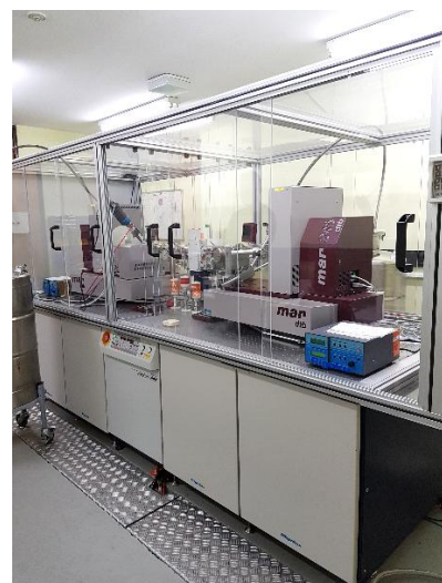
MicroMax™-007 HF Microfocus rotating anode X-ray generator with mar345 image plate detector
