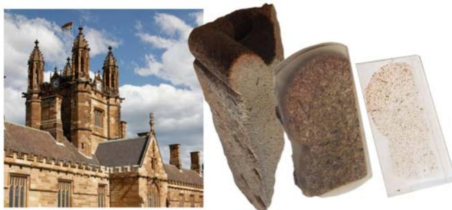
Thin-section made from a sandstone sample collected from the Main Quadrangle, University of Sydney. The porous sample was set in epoxy before mounting on a glass slide.
