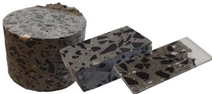
Thick-section (100  $\mu\text{m}$ ) made from a sample of terrazzo flooring used in the new School of Life and Environmental Sciences building.
