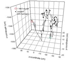
The number of neutrons counted over a period of time is inversely proportional to the amount of water in the soil.
