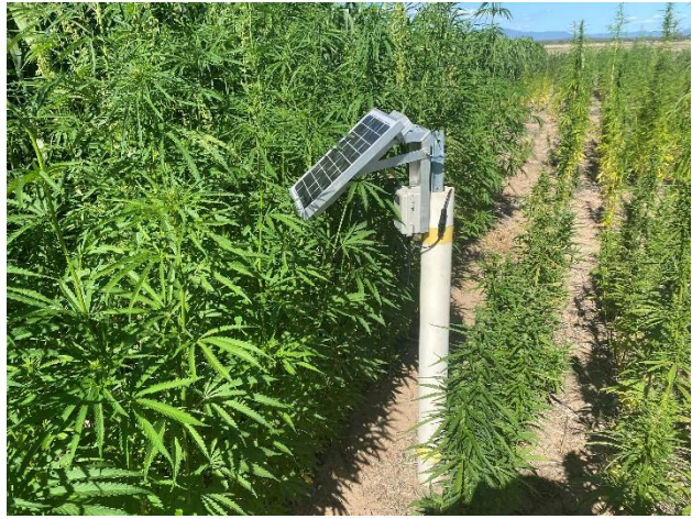
Figure 9: Low THC Hemp trial in January 2023 showing soil probes used to record soil moisture and temperature
