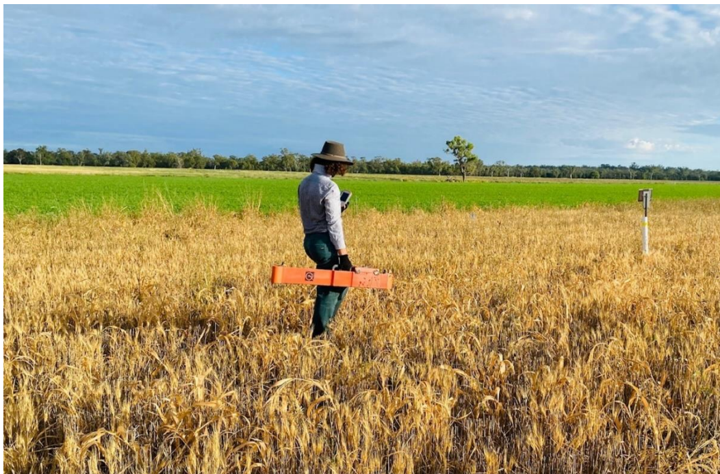
Figure 18: PhD Student Tom O'Donoghue completing his last measurements using an EM to measure soil moisture in January 2022. A soil moisture capacitance probe can also be seen in the background.
