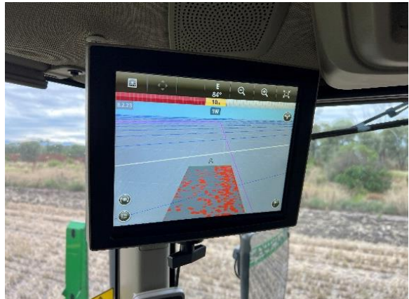
Figure 16: John Deere See & Spray Technology for Precision Weed Management being used for the weed assessment trial – February 2023
