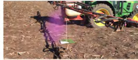
Spray nozzle activates in the vicinity of piece of Astro-turf that was previously mapped using a drone.
