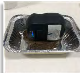
Figure 3. NIRS scanning of wet faecal samples using the handheld NIRVScanTM device
