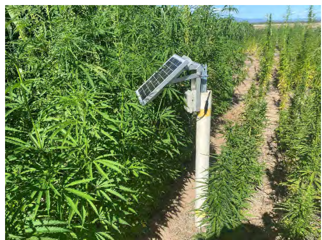
Figure 4: Low THC Hemp trial in January 2023 showing soil probes used to record soil moisture and temperature
