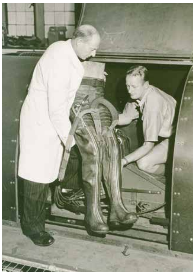
Frank Cotton [in white coat] and assistant Ken Smith load an early model CAAG suit into the centrifuge. The wooden torso and legs survive in the Macleay Museum collection as item 117, or more affectionately, 'George' [Unknown Daily Telegraph photographer] [P147/106]
