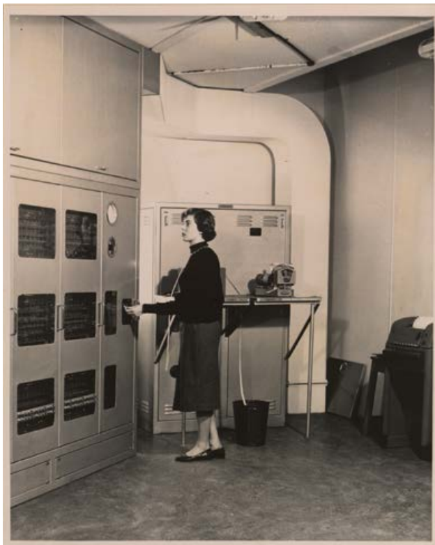
Miss Margaret Ford, research assistant, feeding tape into the tape reader of SILLIAC, 1956. SILLIAC was the University of Sydney's first computer. [1245_1_22]
