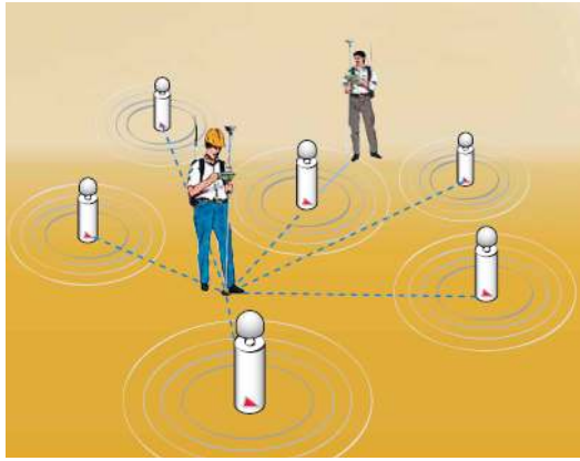
Figure 3. Diagram showing the theory of CORS networks in the field (Leica Geosystems).
