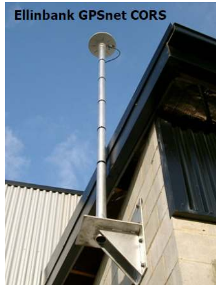
Figure 1. A CORS network base station in the GPSnet network (Hale and Oates, 2009).
