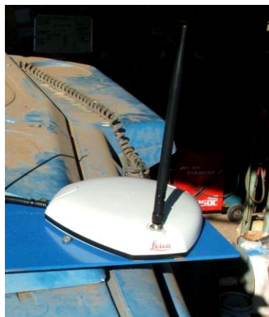
Figure 4. Photo of NextG antennae (black) and GNSS receiver (white) of mojoRTK on tractor roof.
