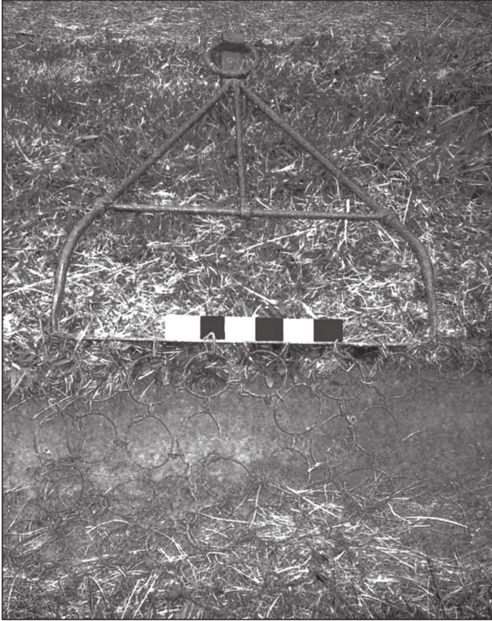
Figure 2.13 An early-style Australian oyster dredge. These dredges were designed to be towed behind a small sail vessel and were used extensively in the Gippsland waterways (scale in 50 mm increments).
