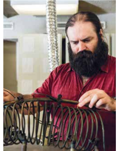
▲ Dr Paddy Neumann checking the coils in a magnetic filter duct that guides and purifies plasma.
